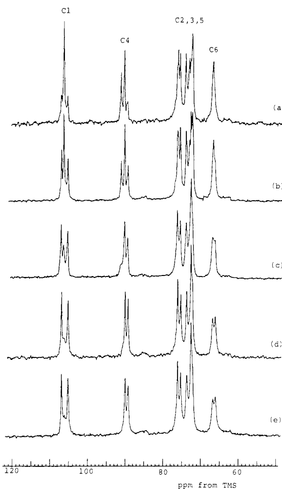
Figure 1. CP/MAS ^{13}\text{C} NMR spectra, 50 MHz, of valonia cellulose treated with steam at different temperatures: (a) original; (b) 230 °C; (c) 245 °C; (d) 260 °C; (e) 280 °C.
